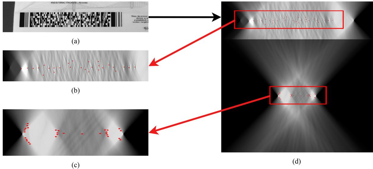
**Fig 4.** The “strongest” points  $\langle P_h, P_v \rangle$  for the source image. (a) Source image  $I$ ; (b) detected  $P_h$  points; (c) detected  $P_v$  points; (d) Sets  $\langle P_h, P_v \rangle$  on the  $FHT$  image
