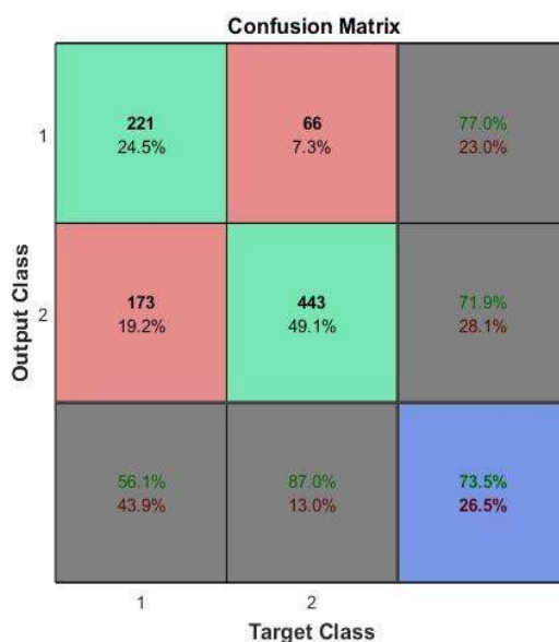
Fig. 8. Confusion matrix of the neural network with a single-layer autoencoder for the Chinese language native speakers (240-50-2)
