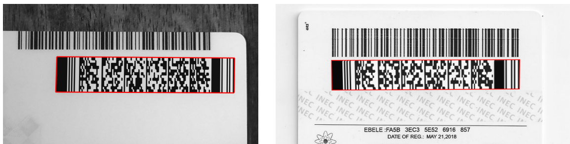
Fig 9. Examples when the quadrangle was found correctly on images containing extra objects
