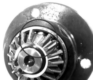
Fig. 5. Pinion with the broken tooth
