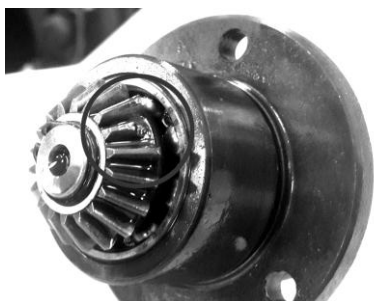
Fig. 4. Pinion with the chipped tooth
