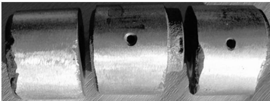
Fig. 4. Flaws of cladded surfaces of cam and its shaft with conventional TIG method
