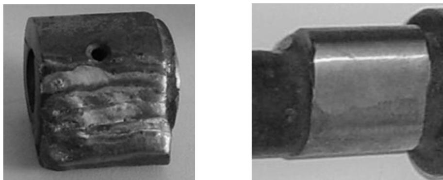
Fig. 5. A general view of surface of cam which remelted and cladded with a high frequency magnetic field TIG-method
