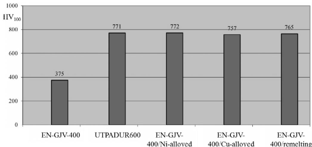
Fig. 10. The hardness diagram of the cladded surface on the cam
