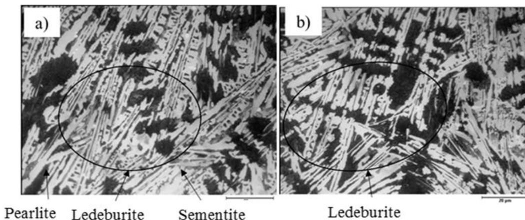
Fig. 11. The microstructure of the copper alloyed cast – iron via TiG (a) and via TiG in high frequency magnetic field (b)
