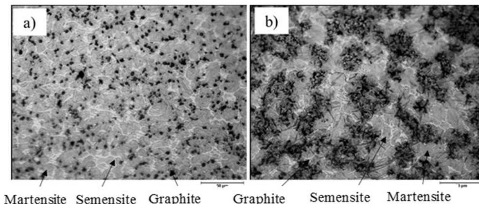
Fig. 9. The microstructure of the nickel alloyed cast – iron via the foil Ni78Si8B14. a – surface alloying via TIG remelting process; b – surface alloying via TIG remelting in high frequency magnetic field
