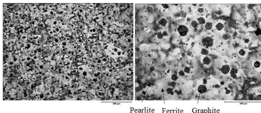
Fig. 6. Microstructure of cast iron EN-GJV-400 grade
