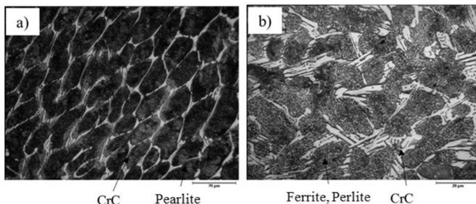
Fig. 7. The microstructure of the surface of the layer UTP A DUR 600 after conventional TIG remelting (a) and TIG remelting in the high frequency magnetic field (b)
