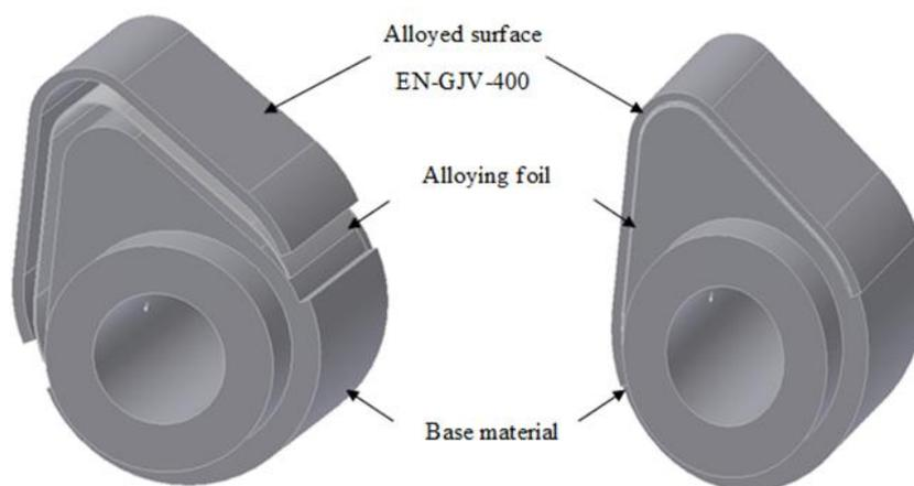
Fig. 3. Schematic description of the surface alloying in high frequency magnetic field
