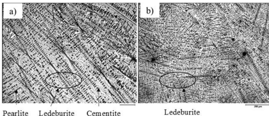
Fig. 8. The microstructure of the layer EN-GJV-400 after conventional TIG remelting (a) and TIG remelting in the high frequency magnetic field (b)
