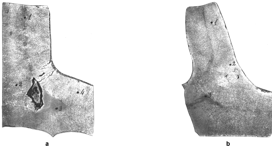
Fig. 2. Macrostructure of two templates (etched with 50 % HCl)
