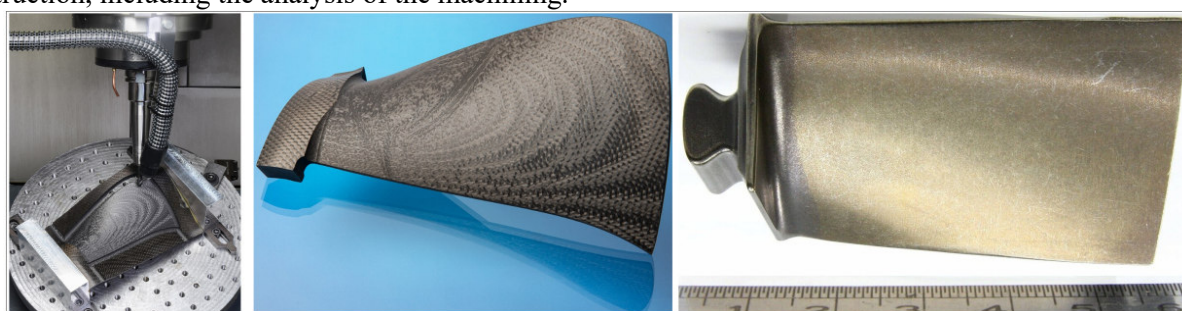
Fig. 1. CNC machining of a fiber-reinforced turbine blade, the machined part (Fraunhofer IPT, 2025) and a similar blade from an enterprise
